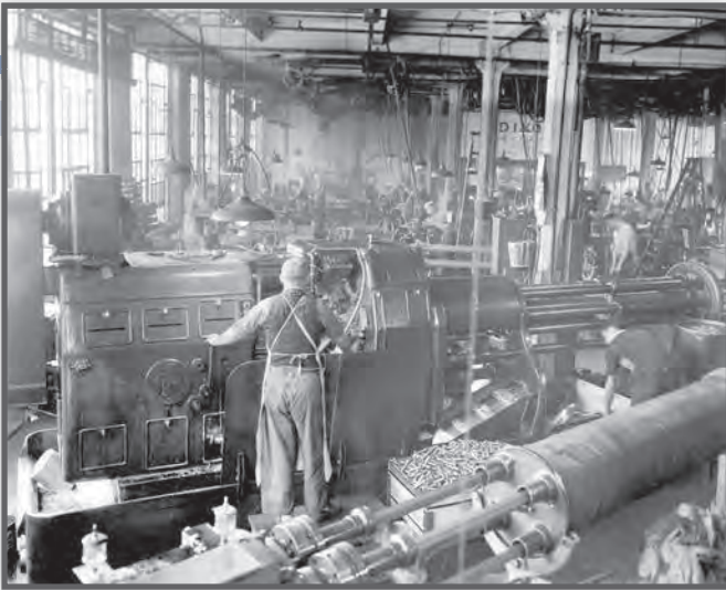
Dixon manufactured fuse plugs to support the WWII effort on a new six-spindle screw machine, the only one in the Philadelphia area at the time.
