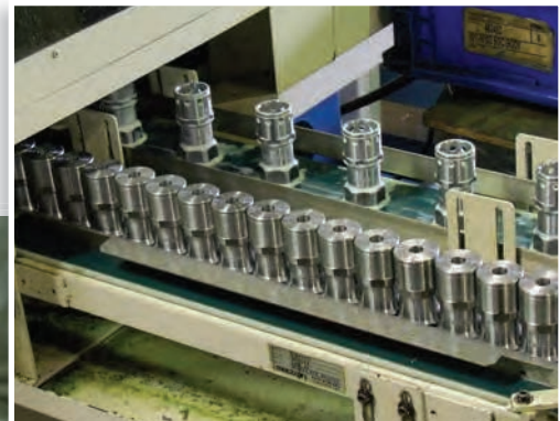
Machining hydraulic couplings at the Quick Coupling plant in Charlotte, North Carolina.
