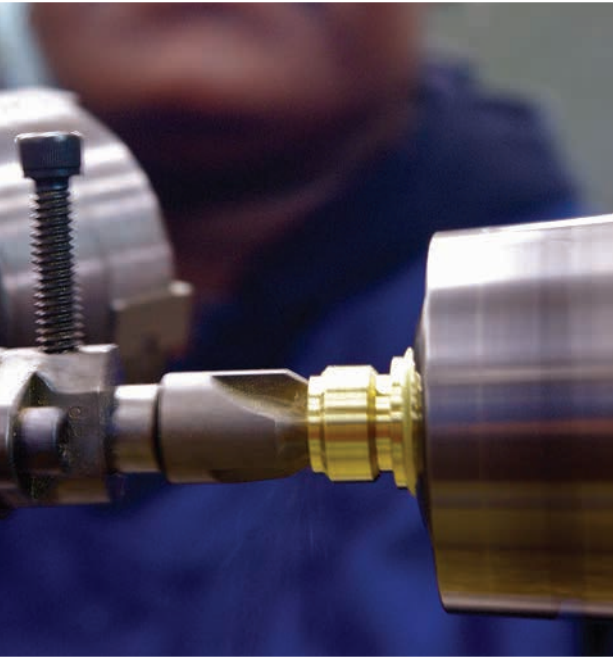
Using a lathe to machine a coupler at the Dixon Brass facility in Westmont, Illinois.
