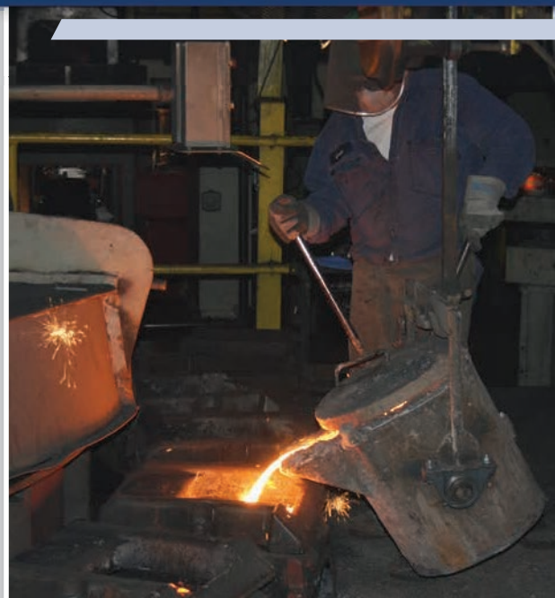
Casting parts at Dixon's Buck foundry in Pennsylvania.
