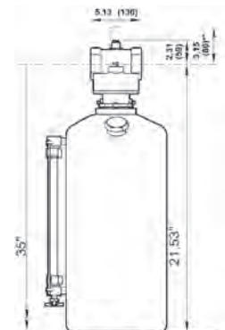
2 and 5 gallon (8 and 20 liter) reservoir ** Optional pyrex sight-feed dome. † Minimum clearance required to remove bowl.
