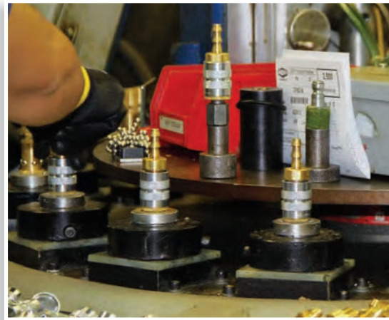
Hand-assembly of an F Series pneumatic coupler.
