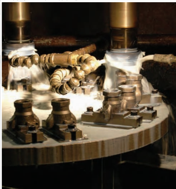
Air King couplers being machined into final products.
